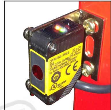
Power on & aligned
